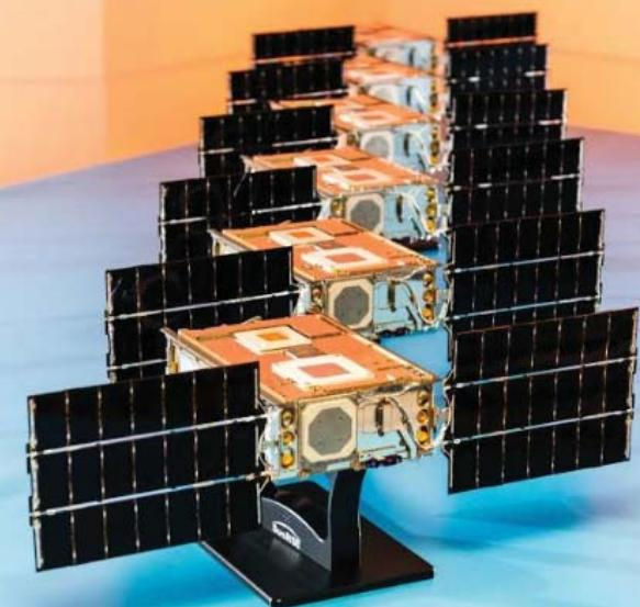
spacecraft electronics -- including on communications satellites in Earth orbit -- and pose a health threat to astronauts. To look out for solar radio events, the SmallSats will fly about 10 kilometres apart and each deploy four radio antennas that extend 2.5 metres. Mission scientists and engineers will track where the satellites are relative to one another and measure with precise timing when each one observes a particular event.
